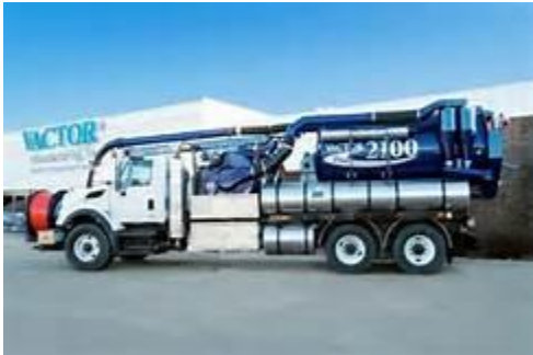
Typical Combination Sewer and Vacuum Truck Used for Sewer Cleaning
